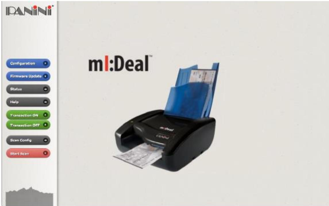
This ml:Deal configuration page will allow you to change the scanner access configuration, update the scanner firmware, check the status of the device and see item capture counts and statistics, access basic information about the device through the 'help' section, review the scan configuration, and perform a test capture from the 'start scan' button.
