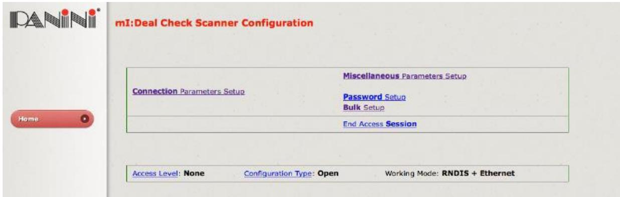
7. Click on Connection Parameters Setup. This link allows configuration of the current access type 'Working mode' for the mI:Deal.
